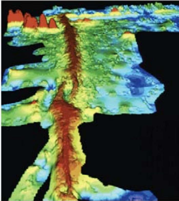
**Figure 3:** Topographic map of the East Pacific Rise showing two long linear volcanoes. Colors are 100m depth contours. The volcanoes are each about 100km long and rise about 300 m above the surrounding sea floor.
